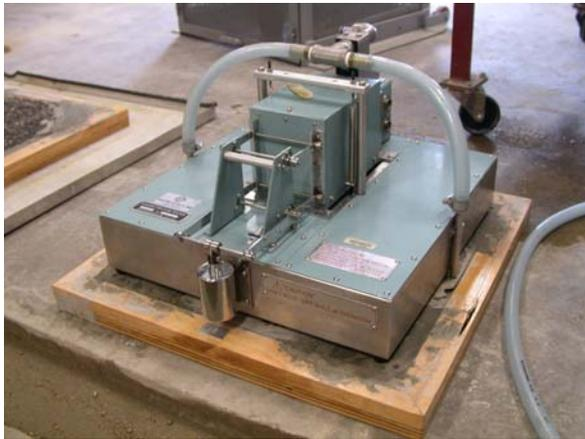
**Figure 2: The DFTester on a Prepared Sample**
